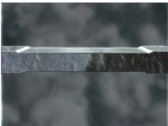
Figure 7. Maximum acceptable embossment that would result from a proper clamping. Dual shiny parallel bands should uniformly extend across the pin on both sides.
