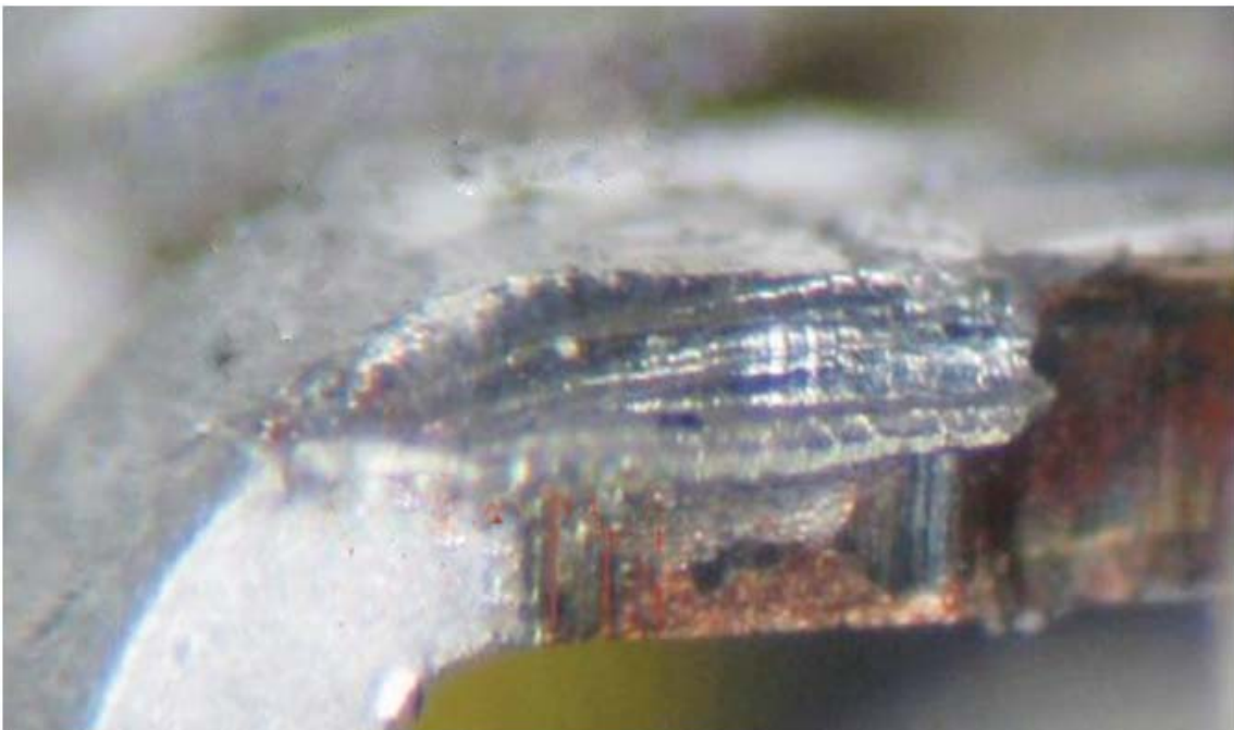
Figure A-1. This image shows the side of a pin which has been hit by an interdigitated comb clamp due to the dambar area being 0.1 mm wider on each side than the nominal pin width, and also because the pins were misoriented (rotated) relative to the comb clamp.
